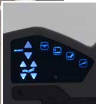
The background lighting increases the patient's self-reliance at night. The function buttons illuminate when touched.
